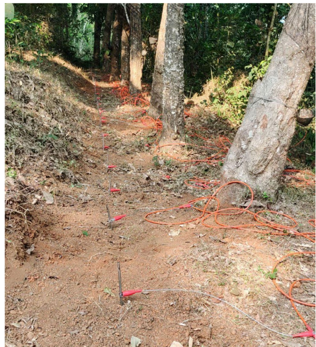
Fig. 7 Typical ERT survey alignment in the field
