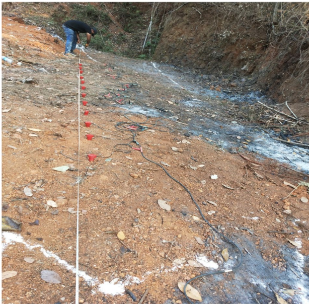
Fig. 8 Typical line 5 of MASW 2D survey
